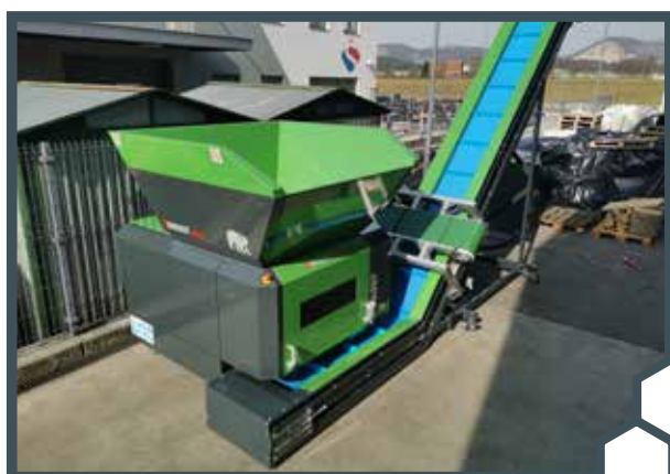
SD90 + RBZ conveyor + magnetic separator
